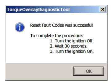
Click 'OK', disconnect the diagnostic program and turn off the ignition for 30 seconds. When you turn the ignition off, you will get the following message:
