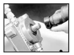
Disconnect column 2. Remove the steering column from the gear input shaft.
