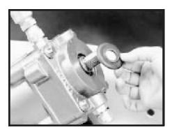
Remove dirt & water seal
