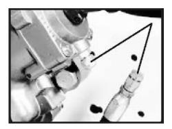
Disconnect return line 1. Disconnect return line from the steering gear and plug the line. Also cap the return port of the gear with a high pressure fitting.
