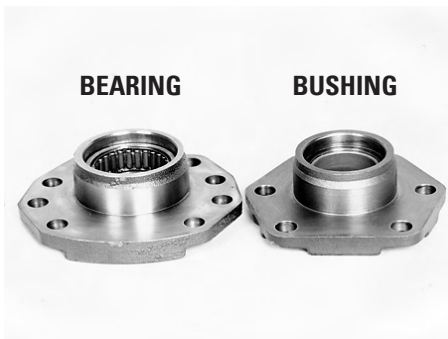
Inspect side cover bushing/bearing
