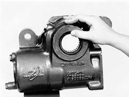
Install dirt seal
