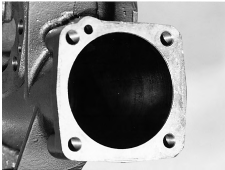
Inspect housing cylinder bore
