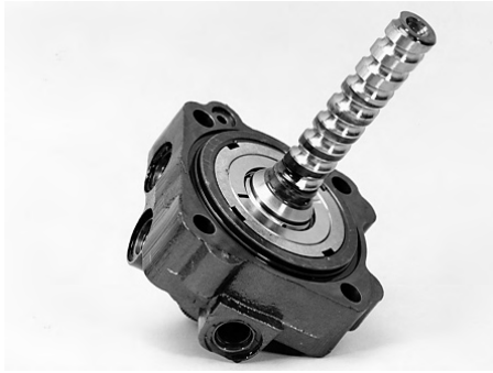
Inspect input shaft, valve/worm assembly sealing areas
