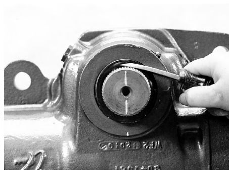
Remove dirt & water seal
