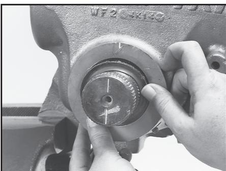
**Remove tape, install dirt & water seal**
