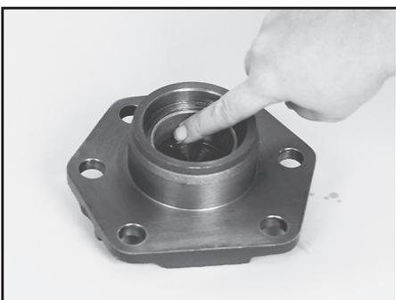
**Lubricate side cover bushing/bearing**
