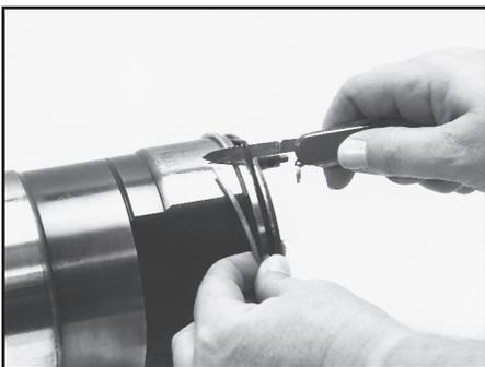
**Remove seal ring and o-ring**
