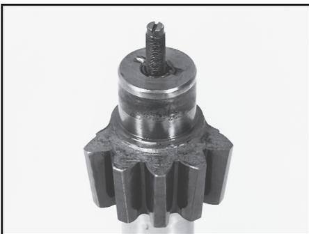
**Inspect adjusting screw and retainer**
