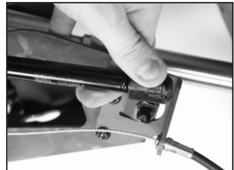
Figure 6 - Install socket End of Gas Spring
