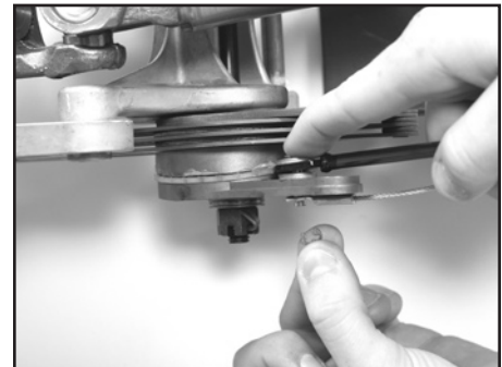
Figure 5 - Secure Clevis Pin
