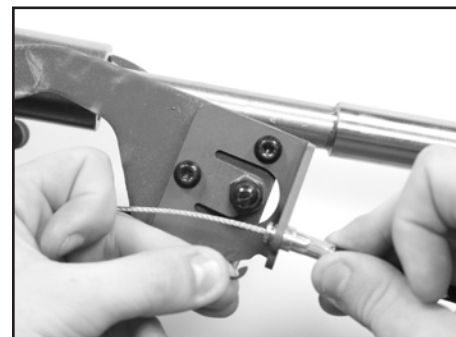
Figure 3 - Install Barrel Fitting
