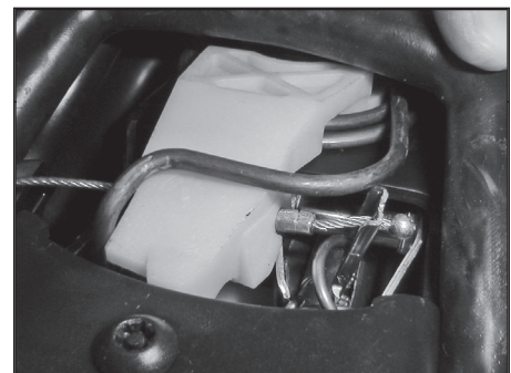
Figure 8 - Cable Assembled to Cam & Tab
