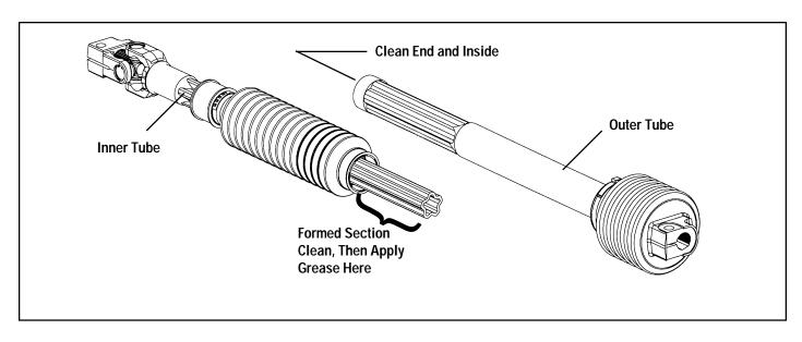
6. Clean the outer tube with a mineral spirits-based solvent. Run solvent into the outer tube and use a soft-bristle brush soaked in solvent to scrub the grease out of the inside of the tube. Also clean off any grease on the outside of the tube.
