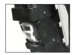
5. Align the tilt lock mechanism holes with the holes in the base unit, and replace the shoulder screw with the threads on the outside of the base unit. Replace the washer and prevailing torque lock nut. Torque the nut to 72-88 lbf•in.
