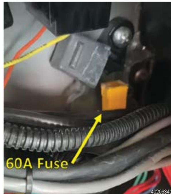
If column power harness does not provide 12V after verifying installation of 60A fuse, contact tech support for assistance.
