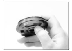
Inspect top plate3. Inspect the top plate (13) for seal area nicks, and abnormal wear or erosion. A polished pattern from the rotor and vanes is normal, grooves you can feel with your fingernail are not normal.
