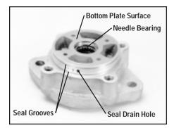
**Inspect cover** 2. Inspect the cover (21) for nicks in o-ring seal grooves. Make sure the seal drain hole is open, and the seal bore is free of nicks and other damage.
