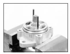
Install locating pins 8. Install the locating pins (18) according to the marks you made on the outside of the housing during disassembly.
