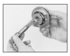
**Remove input shaft** 14. Push the input shaft (7) out of the pressure plate (10).
