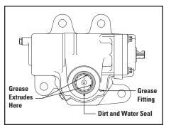
Maintain input shaft dirt & water seal grease pack
