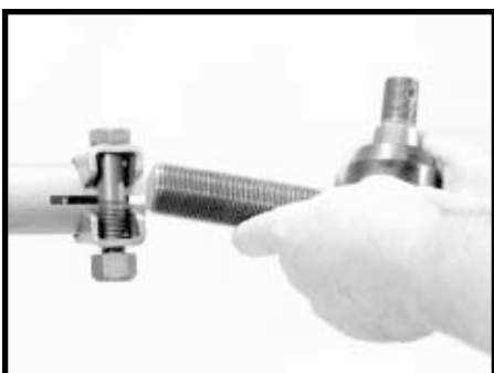
Install new socket
