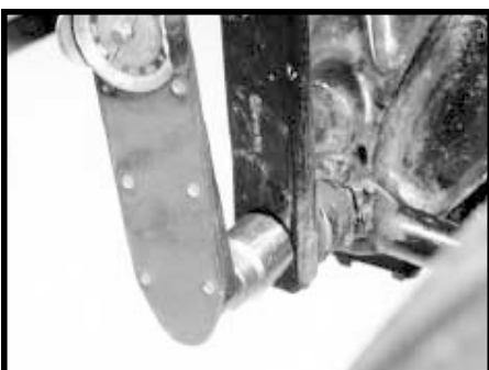
Install new drag link
