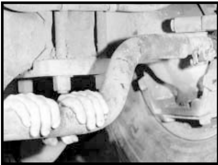
Center tie rod
