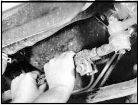
Center tie rod
