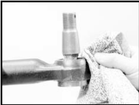
Clean socket area
