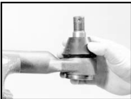
Install new seal
