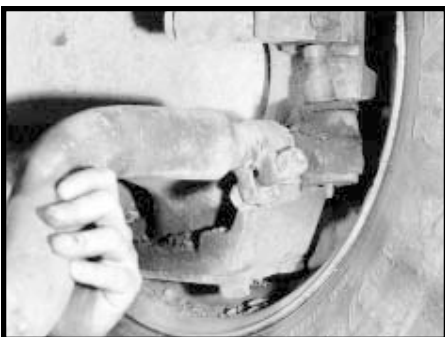
Disconnect tie rod
