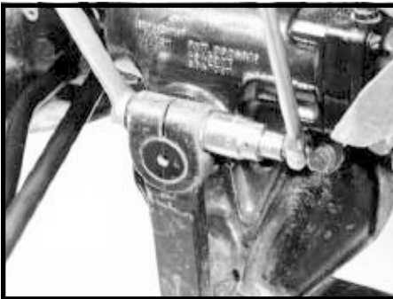
Remove pinch bolt
