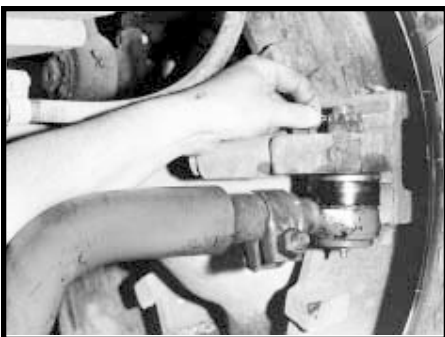
Install new linkage
