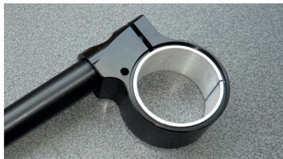
1. To facilitate mounting, apply suitable grease to the conical section of the handlebar stubs (end with thread for clamp).
