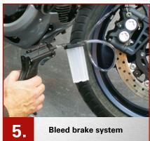
5. Subsequently refill the brake system and bleed it.
