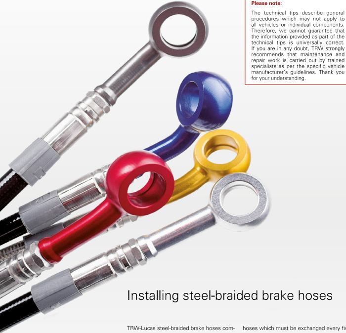
prise a stainless steel mesh in a plastic coating, fitted with an internal PTFE hose. As a result, you will always be on the safe side. Unlike the majority of OE standard rubber parts, TRW-Lucas hoses do not expand under high temperatures or brake pressure and therefore offer an improved brake response and a more precise perceptible pressure point.
