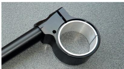
1. To facilitate mounting, apply suitable grease to the conical section of the handlebar stubs (end with thread for clamp).
