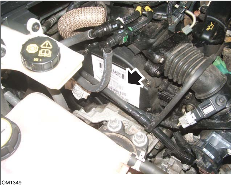
1.6 TDCi Engines: - Injector label arrowed in illustration
