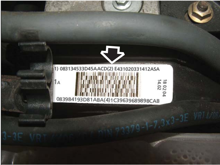
Injector label - gives four 16 digit numbers
