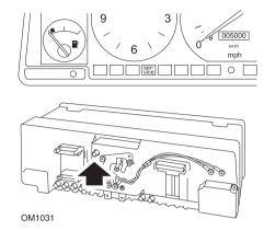
Reach behind the instrument panel and push the button located to the left of the speedometer.
