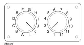
If using the EOBD (J1962) pin-switchable cable (YTD951), ensure the settings on the switch box correspond to the settings listed for the vehicle and system being tested
