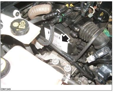
1.6 TDCi Engines: - Injector label arrowed in illustration
