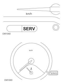
The lamps illustrated above, are Malfunction Indicator Lamps (MIL) and not service interval indicators. When illuminated there is a problem with the vehicle. Refer to manufacturer's documentation for further information.
