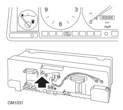
Reach behind the instrument panel and push the button located to the left of the speedometer.
