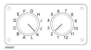
If using the EOBD (J1962) pin-switchable cable (YTD951), ensure the settings on the switch box correspond to the settings listed for the vehicle and system being tested.
