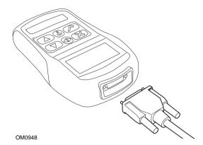
The service tool has a 15-way connector through which it can communicate to the vehicle via various interface cables. Connection to the specific system is via either the vehicle's EOBD (J1962) diagnostic socket or by a system specific connector. Refer to the 'Vehicle Application List' to determine the correct cable.
