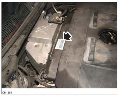
2.0 TDCi Engines: - Injector label arrowed in illustration - Side view
