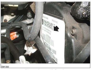
Injector codes arrowed in illustration
