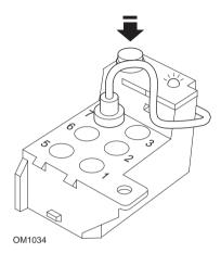
Diagnostic module located in engine compartment adjacent to LH suspension mount
