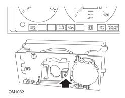
Reach behind the instrument panel and push the lever located between the tachometer and the speedometer.
