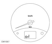
The lamp illustrated is an oil level low warning indicator and not a service interval indicator. When the engine oil is at the correct level, this lamp will automatically extinguish.
