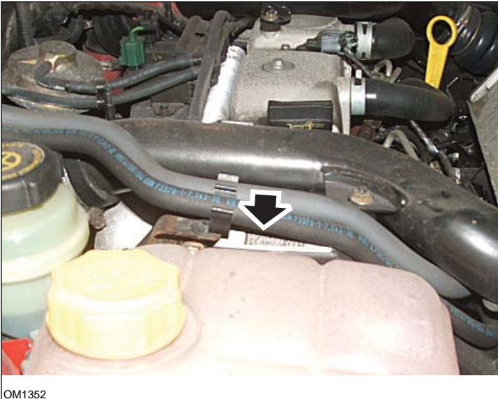
1.8 TDCi Engines: - Injector label arrowed in illustration - Side view
