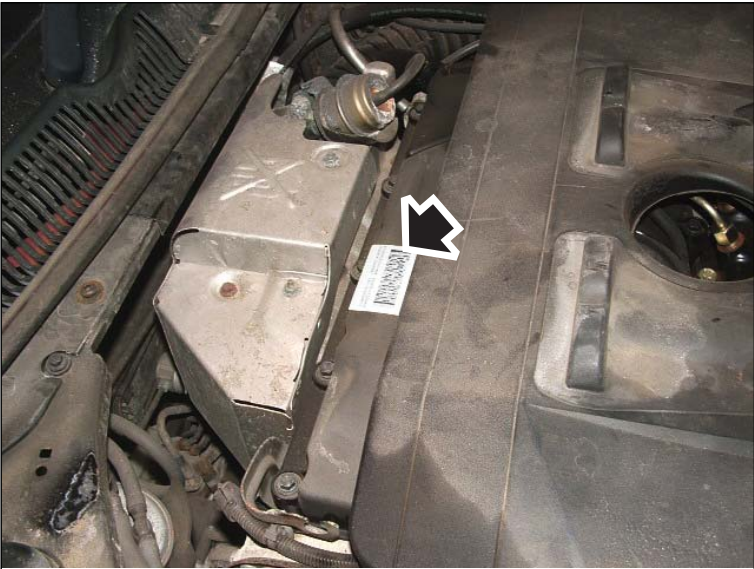
2.0 TDCi Engines: - Injector label arrowed in illustration - Side view
